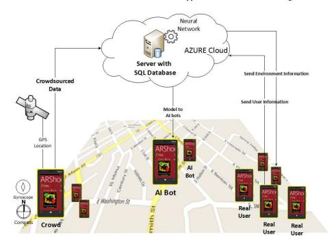
**Fig. 2.** The proposed architecture. The crowd contributes spatio-temporal information to the server on the clowd (left). The server uses the crowdsourced data to train AI agents that are deployed in the game's environment (center). The real users exchange information with the server regarding their location, the opponents' locations, health etc. (right)
