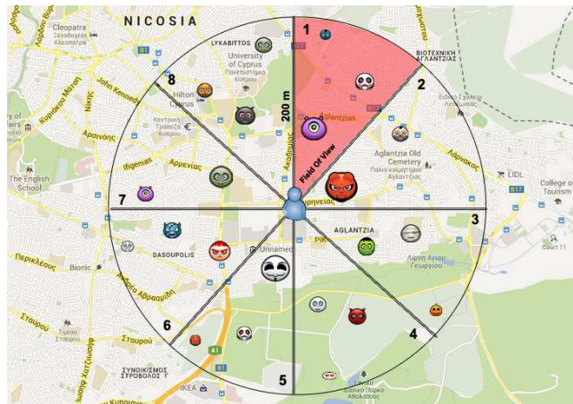
Fig. 1. The surrounding environment of the players is split into eight sectors in order to collect spatio-temporal information. The closest opponent's avatar is to the user, the larger appears in the augmented reality view.
