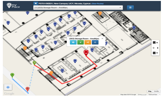
Fig. 5. The AnyPlace Indoor Information Service (screenshot relates only to the Web Viewer) facilitates the task of crowdsourcing models, context and radiomaps for indoor spaces but also supports intelligent search and navigation in buildings uploaded publicly or privately.
