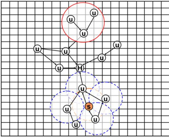
Fig. 7. Example of a network design  $X$  with sensors  $u$  not satisfying conditions C1, C2, C3 and the shadowed sensor  $s$  being eligible for relocation. The dashed circles indicate the sensors'  $R_s$  and the solid circle indicates an example of a possible network partition.
