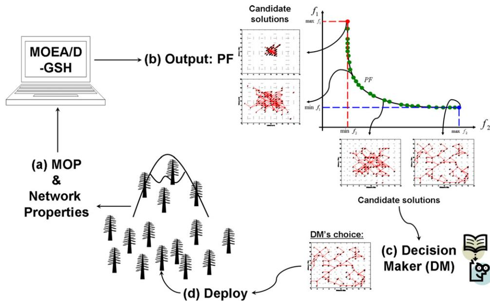
Fig. 18. MOEA/D-GSH as a sensor placement tool in a monitoring information system for fire detection applications in forests.
