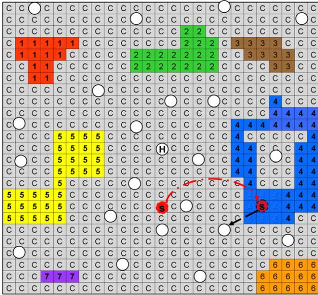
**Fig. 10.** The main concept of  $ImpCv_2(X)$ . The network design is divided into  $\psi = 7$  coverage holes  $\Psi_j$ , where  $j = 1, \dots, 7$ . The covered grids are denoted as  $c$ . The sensors are marked as circles. Sensor  $s$  satisfies all conditions  $C_1, C_2, C_3$  and is relocated within the largest coverage hole, i.e.  $\Psi_4$ , to cover a previously uncovered area (shown as embossed 4).
