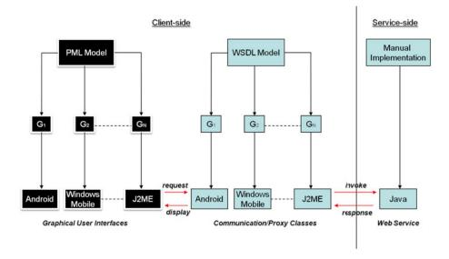
Fig. 1. Model-Driven, Web Service-oriented Architecture
