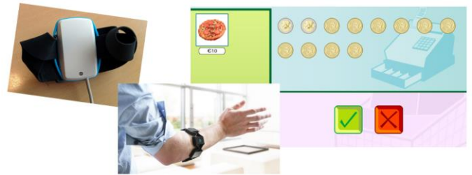
Figure 8. Controlling the EURO application with simple wrist movements - for people who are not able to control their hands or feet with precision.
