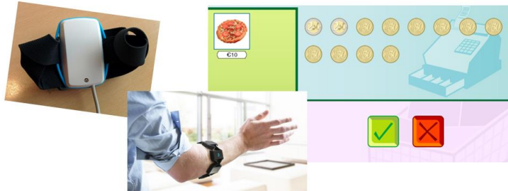
Fig. 8. Controlling the EURO application with simple wrist movements - for people who are not able to control their hands or feet with precision.
